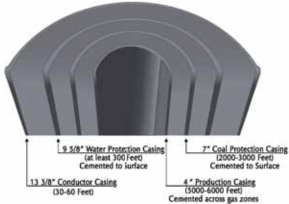
*Fresh water in Virginia is generally less than 300 feet deep. Rock formations containing natural gas are several thousand feet to more than a mile deep. Several casing strings are cemented to surface to isolate natural gas from contacting fresh water sources as illustrated in the diagram at left and above.*
